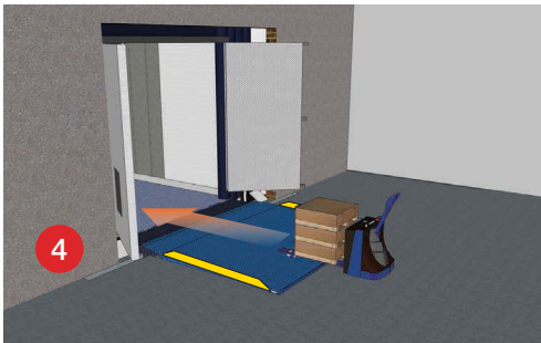
Loading and unloading process takes place like a standard pit-mounted leveler.
